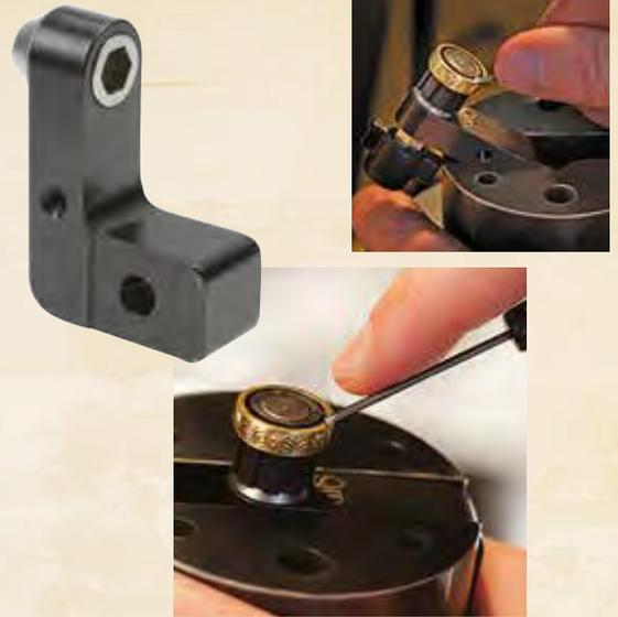
Get better clearance when engraving the outer side or circular edge of rings with this outside frame assembly. The assembly can be kept in place at various angles in a vise. The set screws which help to hold it in the vise can also be removed for greater freedom of movement.
