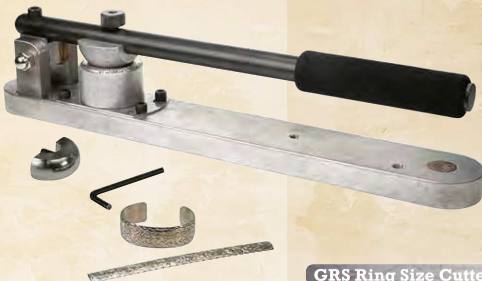
Easily shape "C" style bracelets with the GRS Bracelet Former. Form flat strips of metal to a perfect "C" shape after engraving the design. The die cup contains a soft alloy material that supports pressure from the die, but does not distort engraved work. The die cup material can be reformed by heating, when necessary.
