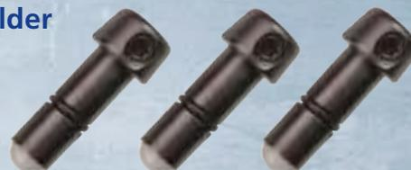
Change the impact characteristics of GRS handpieces just by mounting a tool or graver in these new Soft-Hit QC Tool Holders. These give a softer impact because the back end of the tool holder is made with a special plastic tip. This creates a smoother, softer energy transfer from the handpiece piston to the tool.
