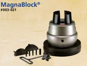
The MagnaBlock provides additional stability while using power tools, chasing hammers, and similar equipment. A massive ball-and-roller bearing system allows smooth rotation without wear or looseness. The internal rotational brake system allows the user to easily adjust rotational resistance. Machined from solid stainless steel with a satin finish and black jaws to reduce glare and eye strain.
