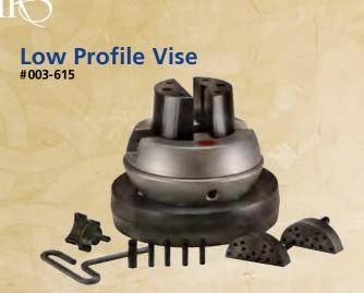
Find just the right working height under a microscope with this vise. When a workpiece calls for a lower height, the Low Profile vise provides a comfortable 152 mm of space for a proper view and position. This vise has the same jaw size and capacity as the MagnaBlock, yet is 38 mm shorter. Top half of vise rotates while bottom half remains stationary. Add the Turntable Base (#003-616-V2) for whole vise rotation.
