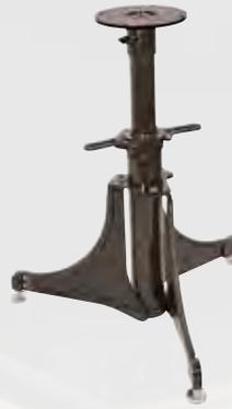
Artists appreciate the Satellite Turntable Stand for the maximum ease of movement and the ability to work on larger pieces. The stand adjusts to ideal working heights between 46 and 73 cm. Its gas spring mechanism and integrated chuck make adjusting quick and effortless. The tripod base provides for incredible stability and the successful completion of even the most intricate cuts. The Satellite Turntable Stand is compatible with the
