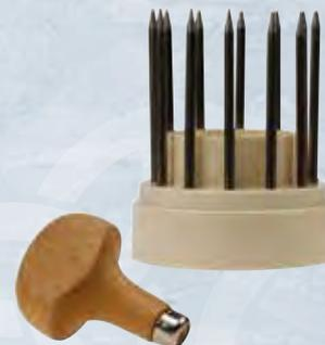
Hardened concave steel tools for forming beads around stones or making dot backgrounds. Set includes twelve beading tools: Size 2, 4, and 6 – 16. Tool #16 makes a 1 mm bead or dot. Tool size increases 0.05 mm.
