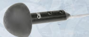
This GRS Burin is a special tungsten carbide graver made for hand engraving, especially intaglio print-making. The material is GRS C-Max, a grade of carbide that has the ability to hold a sharp edge for an incredibly long time. Because this material is a very hard tungsten carbide, it can only be sharpened using a diamond abrasive. The burin is made from a 3.17 mm diameter round blank approximately 75 mm long.
