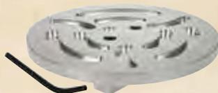
Originally designed to assist the scrimshaw artists at the GRS Training Center in holding ivory panels for engraving, this unique tool uses modeling clay or Thermo-Loc that can be pressed into the milled slots to gently hold a workpiece without damage. Perfect for detailing thin, light pieces that cannot be held by themselves in a ball vise.
