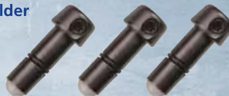
Change the impact characteristics of GRS handpieces just by mounting a tool or graver in these new Soft-Hit QC Tool Holders. These give a softer impact because the back end of the tool holder is made with a special plastic tip. This creates a smoother, softer energy transfer from the handpiece piston to the tool.
